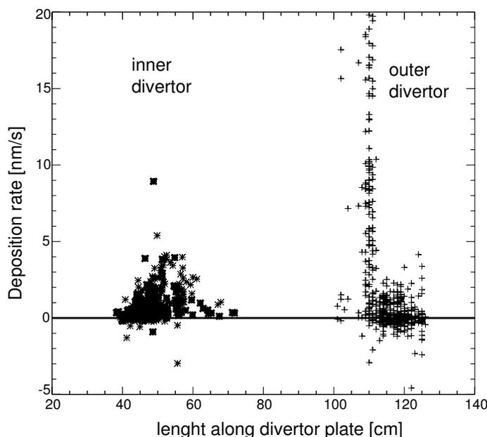
**Fig.2:** Deposition rate at the inner and outer divertor during the 2003 experimental campaign measured by the QMB C (\*) and QMB B (+) respectively. The x axis corresponds to length along the divertor plates (Fig. 1)
