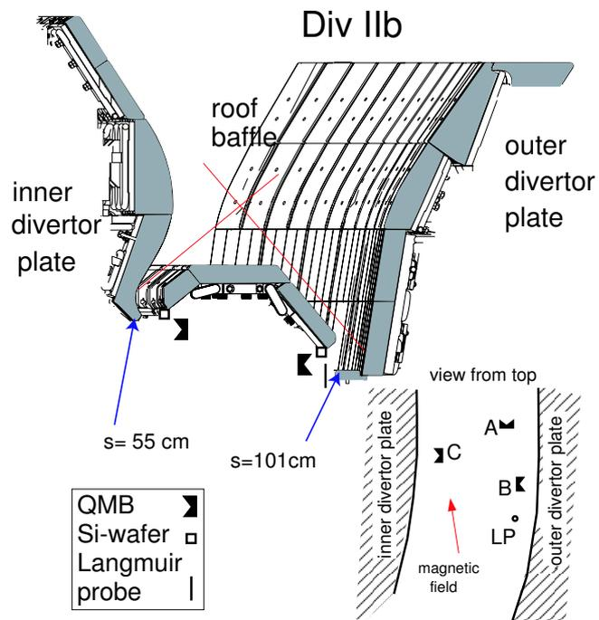
Fig.1: Position of the QMB monitors below the roof baffle of Div IIb at ASDEX Upgrade.
