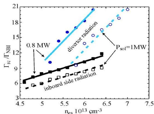
Figure 4: Neutral gas penetration flux into the core as a function of  $n_{es}$ ,  $P_{sol}$  and configuration calculated by the 3D code.
