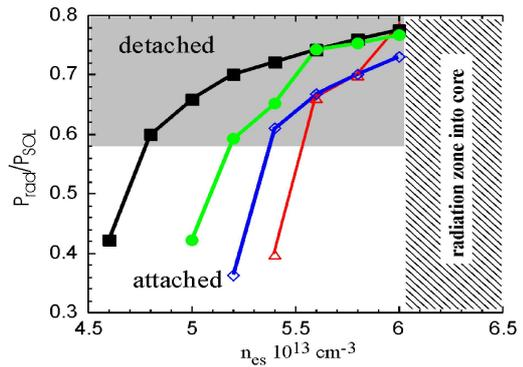
Figure 2: Carbon radiation normalized to  $P_{sol}$  as a function of  $n_{es}$  and configuration.
