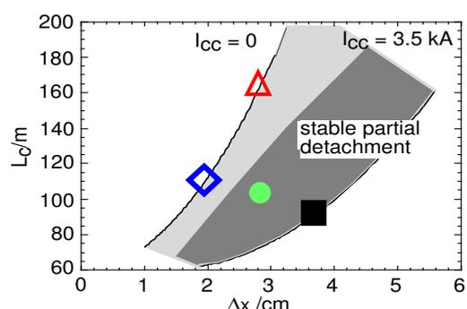
Figure 1: Stable partial detachment is restricted to large  $\Delta x$  and small  $L_c$  ranges (shaded region). Four configurations are selected for numeric studies.
