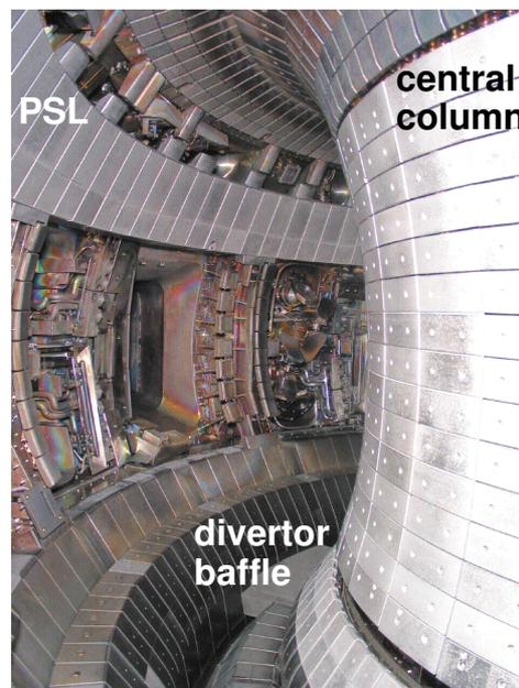
**Fig. 1:** *View into ASDEX Upgrade. During the campaign 2002/2003 the complete heat shield (HS), the upper passive stabiliser loop (PSL) and the inner divertor baffle (DB) have been covered with new tiles coated by W.*
