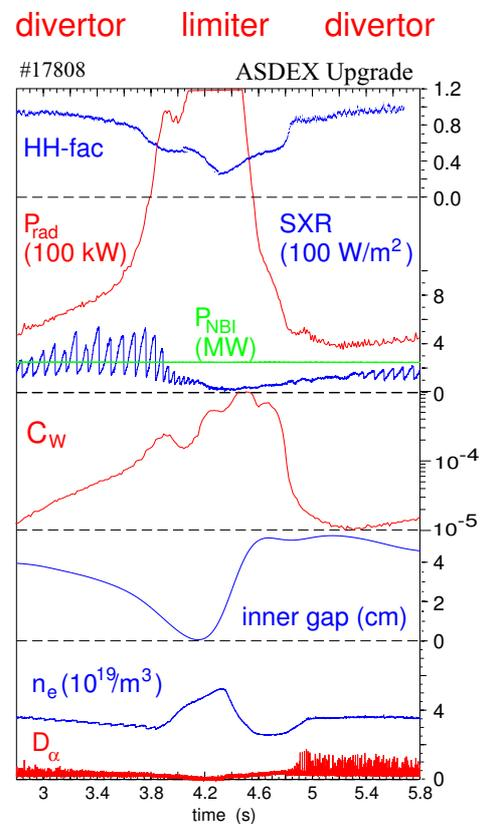
**Fig. 4:** Plasma parameters during a transition from divertor to limiter and back to divertor operation induced by a scan of the inner gap for a  $I_p = 1$  MA,  $B_t = -2.4$  T discharge.
