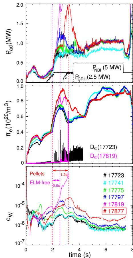
**Fig. 3:** Temporal behaviour of plasma parameters in standard-H-mode discharges for different states of machine conditioning. In #17877 80Hz pellets were injected from 2.0-3.2 s
