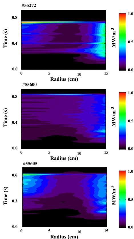
Figure 3: Time evolution of radial profiles of radiated power in a 1 MW NBI divertor plasma above the density threshold with  $B = 2.5$  T in D (top), H (middle) and H with N puffing (lower). N puffing begins at 0.25 s.
