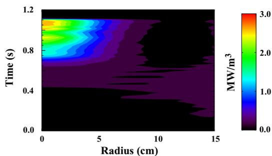
Figure 2: Time evolution of radial profiles of radiated power in a 1 MW NBI divertor plasma at the density threshold with  $B = 2.5$  T in hydrogen. See #55595 in Fig. 1.
