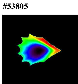
Figure 4: Tomographic reconstruction in the triangular plane of radiated power in a 1 MW NBI partially detached divertor plasma with  $B = 2.5$  T in hydrogen.
