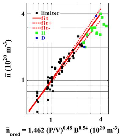
Figure 5: Comparison of achieved and predicted values of line integrated densities,  $\bar{n}_e$ , for density limit discharges in divertor and limiter configurations.
