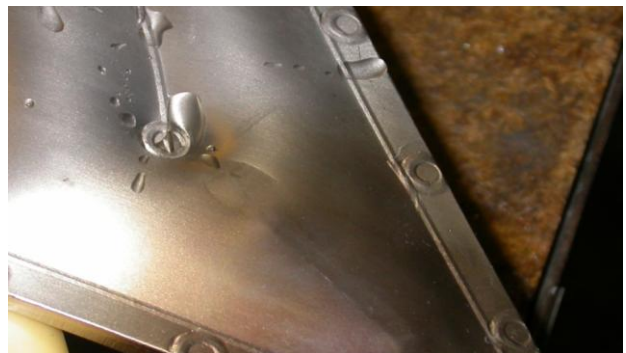
Fig. 4: Failed welding seam at 11 MPa internal pressure
