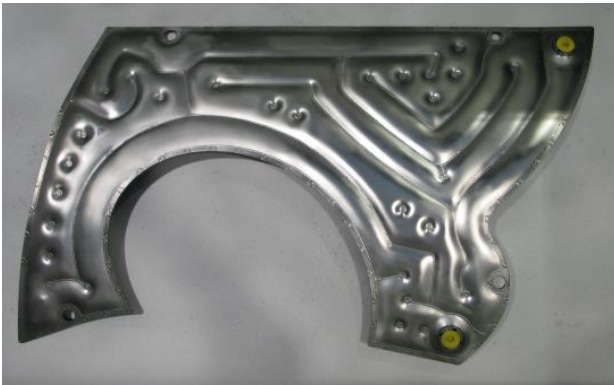
Fig. 1: A typical panel shown from the side opposite the plasma with a large cut-out for a port.
