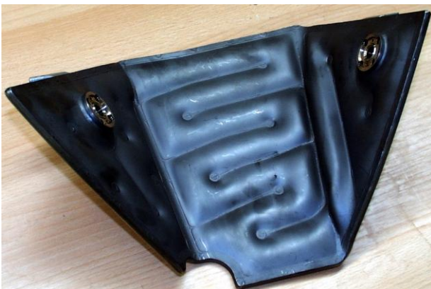
Fig. 3: Panel of the type TP-H003, after burst test.
