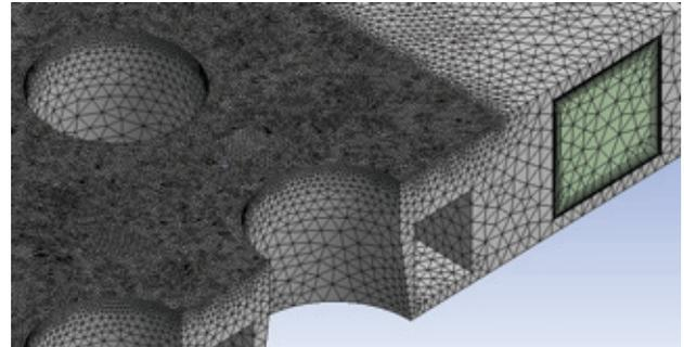
Figure 6 EG Model meshed in ANSYS CFX.
