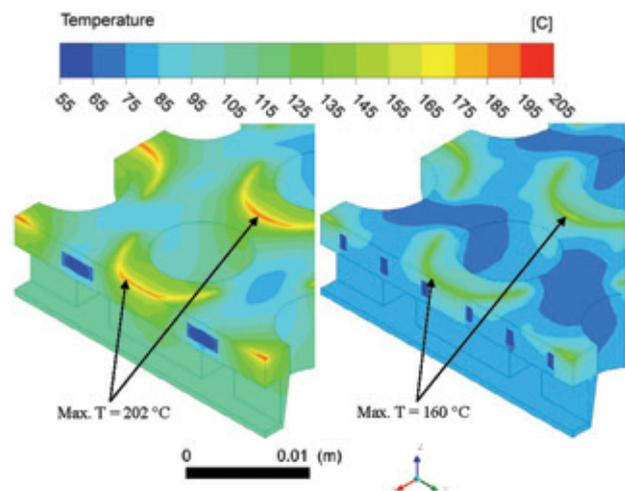
Figure 8 Temperature distribution in SINGAP (left) and ELISE (right) for EDF and FF in orthogonal configuration.
