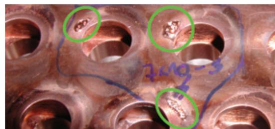
Figure 1 Extraction grid of BATMAN experiment damaged by co-extracted electrons
