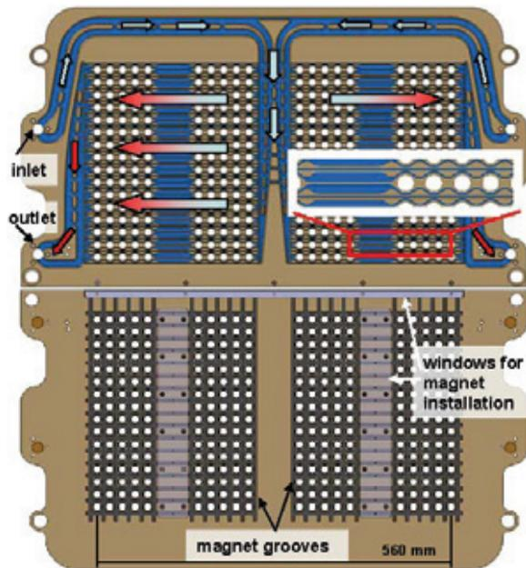
Figure 5 ELISE EG. Upper segment: cooling circuit. Bottom segment: magnet grooves in the back side of the EG, for both EDF configuration.
