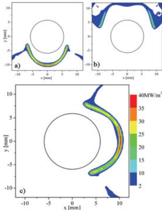
Figure 3 Power density deposition by co-extracted electrons (for 10 kV acceleration and  $30 \text{ mA/cm}^2$  current density) for EDF parallel to FF in subtracted (a) and added (b) fields, and for EDF orthogonal to FF (c).
