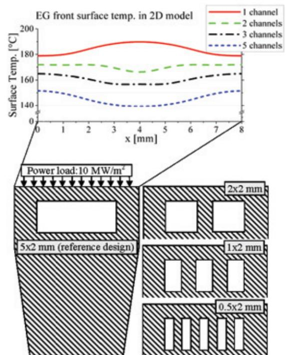
Figure 4 Temperature distributions on the front surface of the EG model for the four different cooling channel geometries
