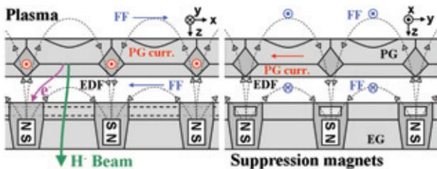
figure 2 parallel (left) and orthogonal (right) configurations of EDF with respect to FF with ion and electron trajectories schematically represented.
