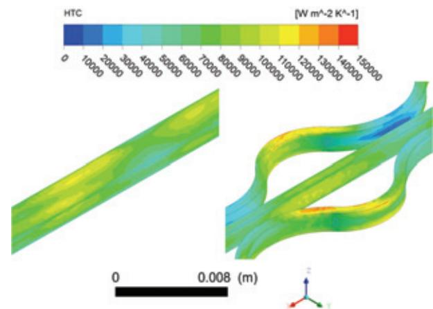
Figure 7 Heat transfer coefficient distribution in EG cooling channels for SINGAP (left) and ELISE (right), EDF and FF in orthogonal configuration.
