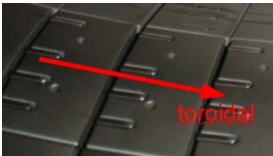
Figure 4: Langmuir probe tips in the outer lower divertor. They are flush mounted in the target tiles and made of tungsten.
