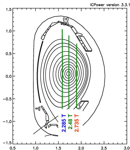
**Fig.1.** ASDEX Upgrade poloidal cross section with H (or 2<sup>nd</sup> D) resonance positions for  $B_0=2.48, 2.285,$  and  $2.735\text{T}$
