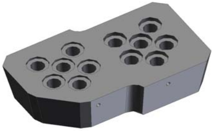
Fig.4. CAD model of the mono-block bridge for the maximal expected shift of adjacent coil blocks.
