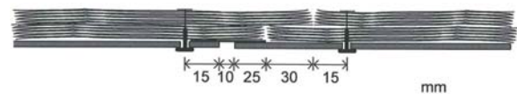
Fig. 3: MLI overlap between the two neighboring panels. Two blankets are shifted against each other.
