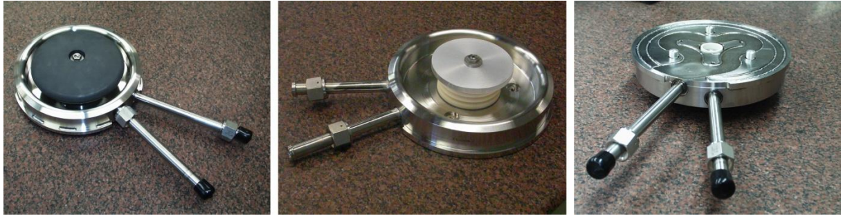
Figure 2: The W7-X glow electrode: top, inside and bottom view.
