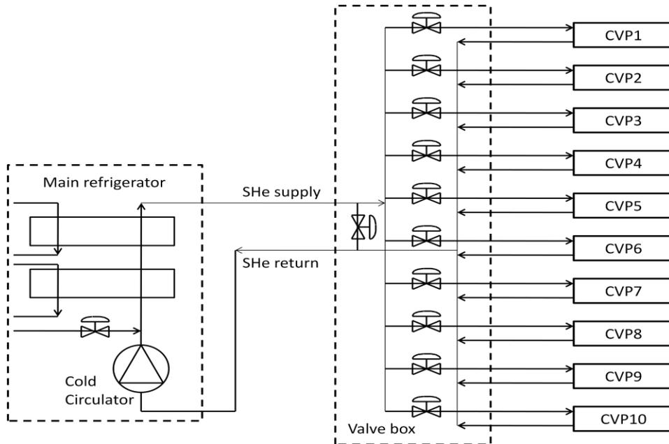
Fig.3 He panel cooling scheme with parallel supply of SHE
