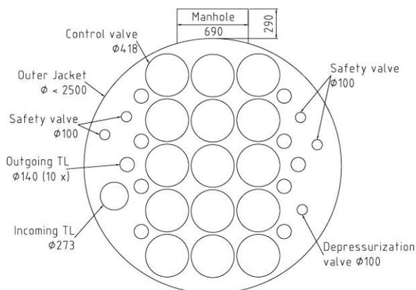
Fig.5 Top view of CVP valve box
