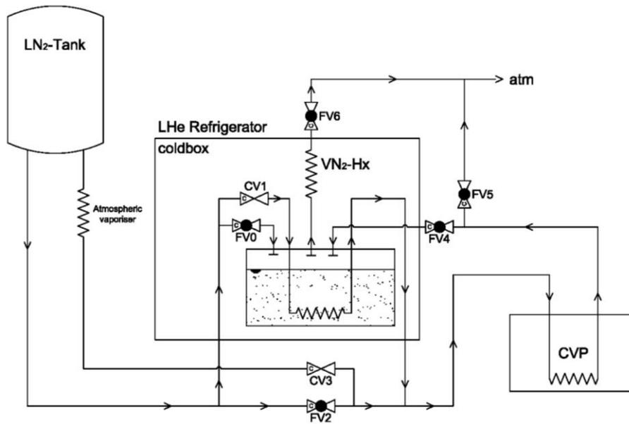
Fig.4 2-phase LN2 cooling scheme of CVP.
