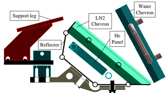
Fig.2 Main components of a CVP
