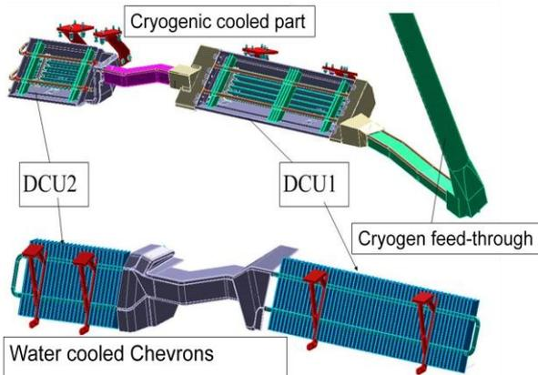
Fig.1 Layout of CVP consisting of DCU1 & DCU2
