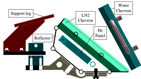
Fig.2 Main components of a CVP
