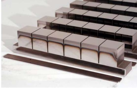
**Figure 1.** Carbon deposition in the gaps of the castellated limiter exposed in TEXTOR
