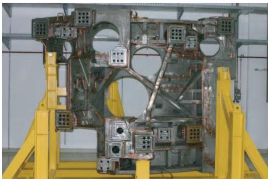
Fig. 3 First segment of the central support ring (1/10 of the full ring). Clearly visible are the cast extensions with the contact surfaces for fixing the coils. The circular holes in this structure are required for the ports on the inner side of the torus.
