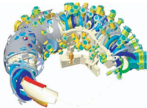
Fig. 1 Cutaway of a CAD drawing of W7-X showing the plasma and the divertor plates (lower left), the magnetic coils around the plasma vessel with inner support structure (upper right) and the Outer Vessel (upper left).
