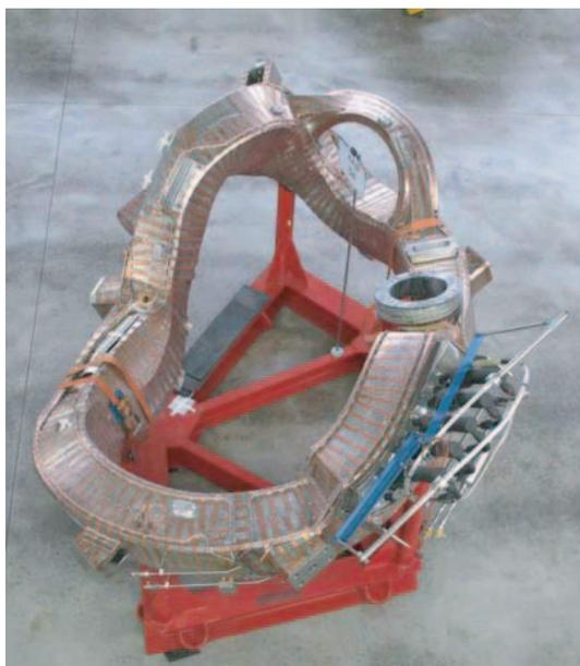
Fig. 2 Non-planar coil type 4 on a transport frame. Clearly visible are the Copper stripes on the coil casing and the cooling tubes. In the lower right part of the picture, the header area with the five interlayer joints and the two superconductor tail ends can be seen.
