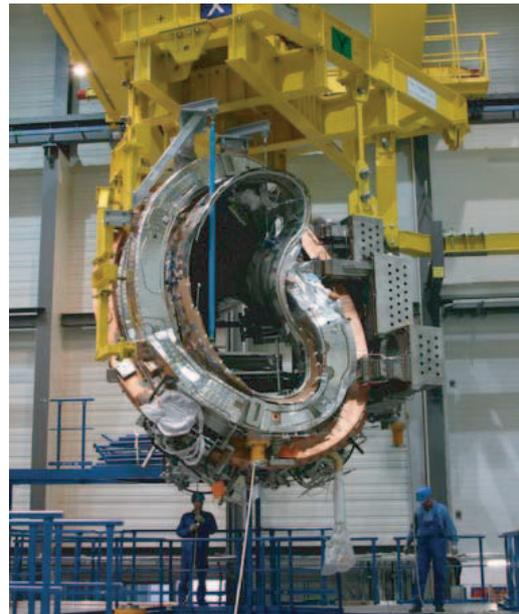
Fig. 5 First magnet half-module being transported to assembly rig II (February 2008). The central support ring with its step flange for connection of the two half-modules is visible on the right as well as the extensions for coil fixation.
