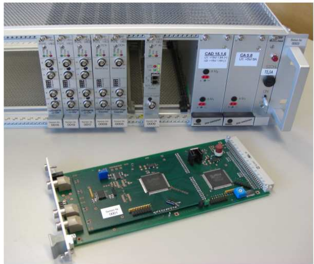
FIG. 6: A photograph of the CPLD based 2-channel phase counter in front of the crate with the 16-bit backplane bus system.
