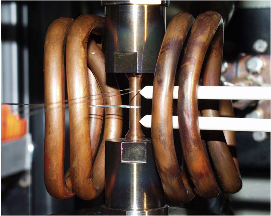
Fig. 2: Measurement of the specimen surface temperature with two thermocouples
