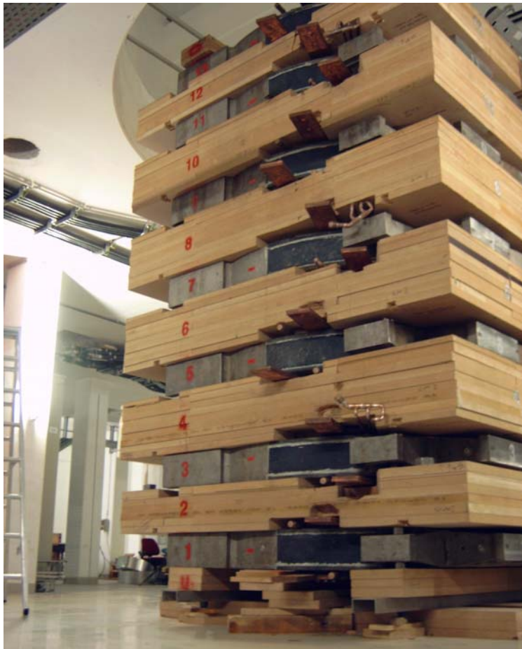
Fig.3: Test loads for the final tests
