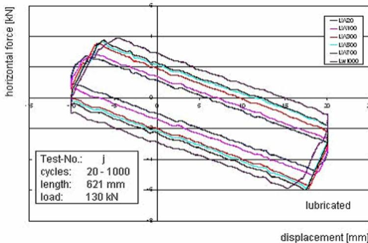
Fig. 6: Horizontal force- displacement- process with a load of 130 kN, cycles: 20 – 1000 [5]
