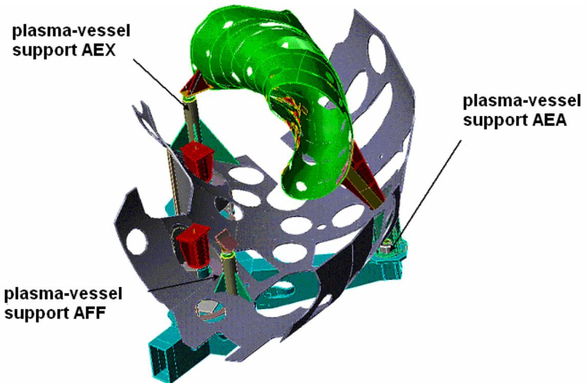
Fig. 2: Half module of plasma vessel with vertical support-devices in shell of outer vessel
