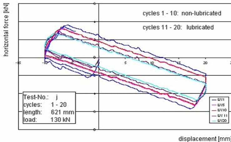
Fig. 5: Horizontal force- displacement- process with a load of 130 kN, cycles: 1 – 20 [5]
