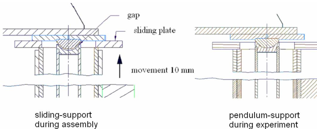
Fig. 3: Schematic view of the pendulum support during assembly and experiment [1]
