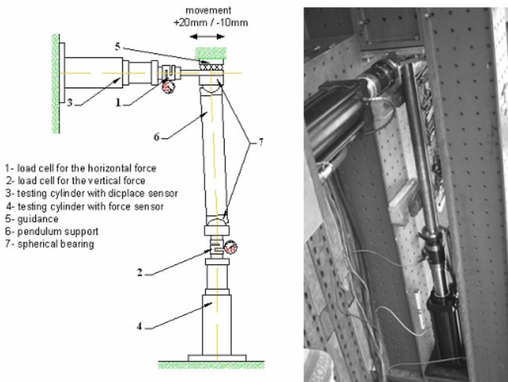
Fig. 4: Principle and original view of the experimental setup
