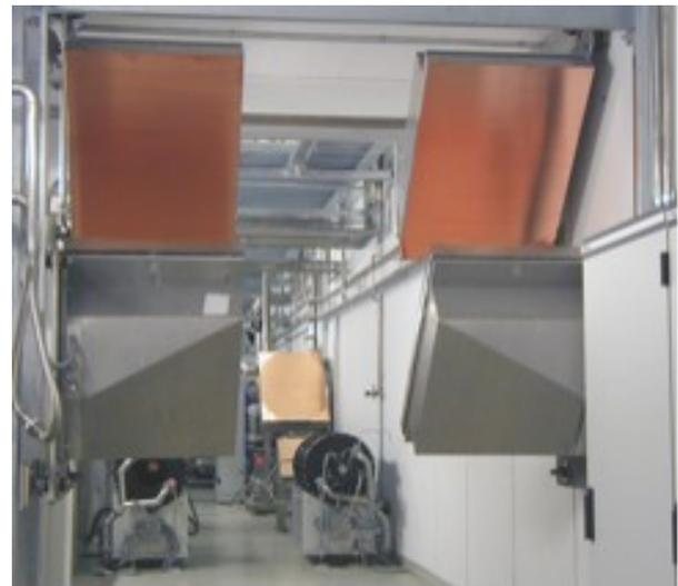
Fig. 13. View into the transmission duct showing mirrors M6, M7 of the two MBWGs (foreground) and the MBWG mirrors M5 as well as mirrors MD, which allows to transmit each individual beam into a calorimetric CW-load (background).
