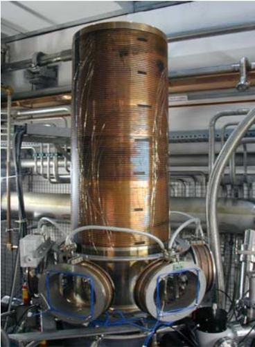
Fig. 10. The TED-gyrotron collector with three pairs of TF-coils (VF-coil removed).
