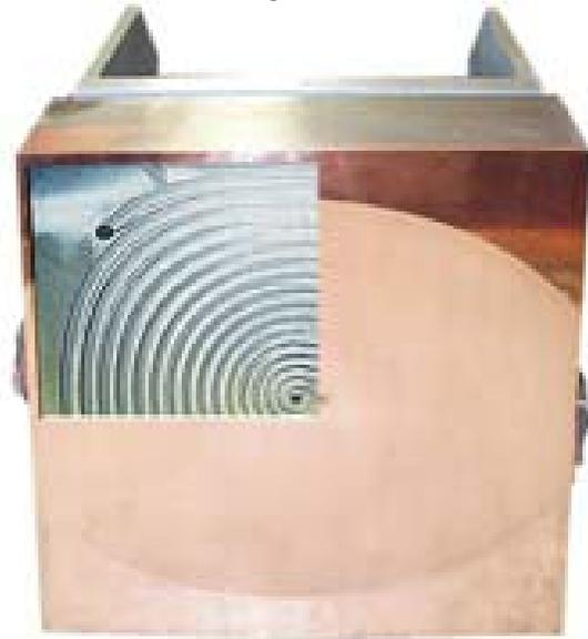
Fig. 15. Single beam mirror with the Cu-SS sandwich structure. The copper surface is partly removed to show the cooling channel.
