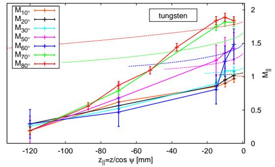
(b) Mach number parallel to the field lines measured by LIF in front of a tungsten target. The dotted lines indicate the predictions of the Chodura model. Their lengths indicate the size of the MPS, respectively.
