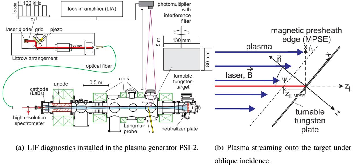
Figure 1: Experimental arrangement
