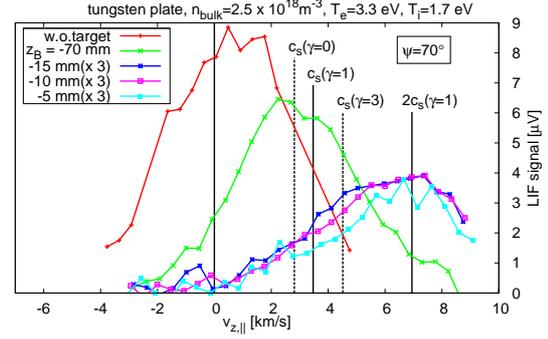
(a) Measured ivdfs at different positions  $z_{||}$  in front of a tungsten target.
