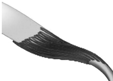
Fig. 5. Poloidally closed drift orbit (here for a 300 keV triton) trapped in the helical mirror of W7-X [24].
