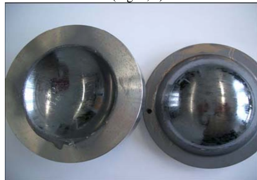
Fig. 8: Test 19/ ball and cup after 1000 strokes
