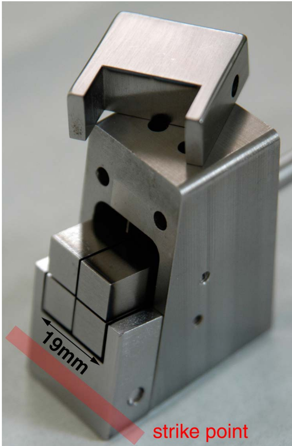
Figure 4: Partially dismantled W gap sample for the ASDEX Upgrade divertor manipulator.
