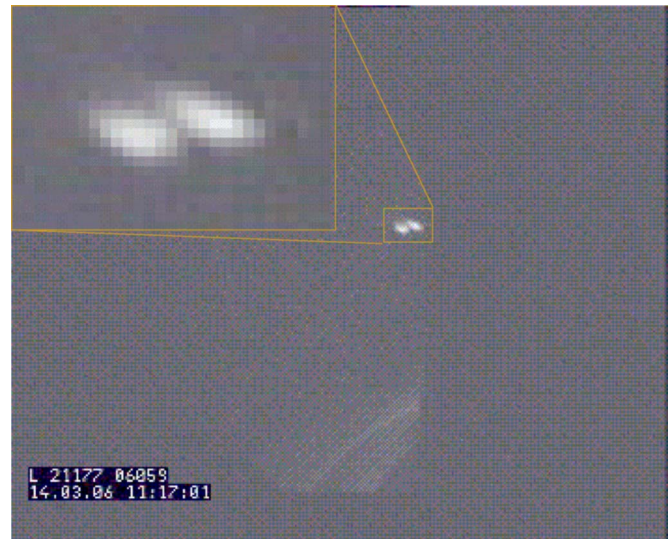
FIG. 6. Video recording (half frame, exposure time 20 ms) of two pellets launched at 100 Hz repetition rate into an ongoing ASDEX Upgrade plasma discharge.
