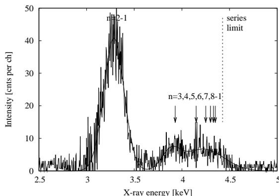
**Figure 1.** X-ray emission for the charge exchange of 39 qeV  $\text{Ar}^{18+}$  ions with an external argon gas target. The black curve marks a fit to the experimental data.
