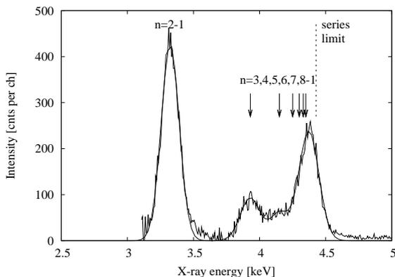
**Figure 2.** *In situ* x-ray emission for the charge exchange of  $\text{Ar}^{18+}$  ions with residual argon gas using a trap depth of 100 V. The black curve marks a fit to the experimental data.
