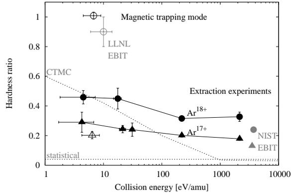
**Figure 3.** Hardness ratios calculated from the x-ray emission spectra as a function of collision energy. Results for capture into  $\text{Ar}^{17+}$  and  $\text{Ar}^{18+}$  are plotted with triangles and circles, respectively. Solid shapes represent extraction measurements and hollow shapes represent those taken *in situ*. Measurements from other groups are marked in grey [6, 7]. The results of CTMC and statistical calculations from [6] are represented by dashed grey lines.
