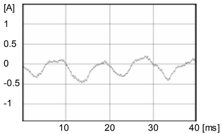
Fig. 2 Measured voltage ripple at 2500 A
