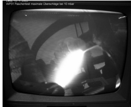
Fig. 8. Camera observation of a breakthrough during a high voltage test under Paschen conditions
