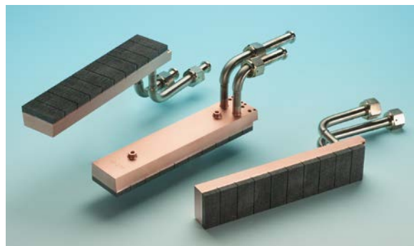
Fig. 1: Elements of manufacturing phase 1. Ten standard top CFC tiles cover the 250 mm long cooling structure. The bent water connectors are used for testing only.
