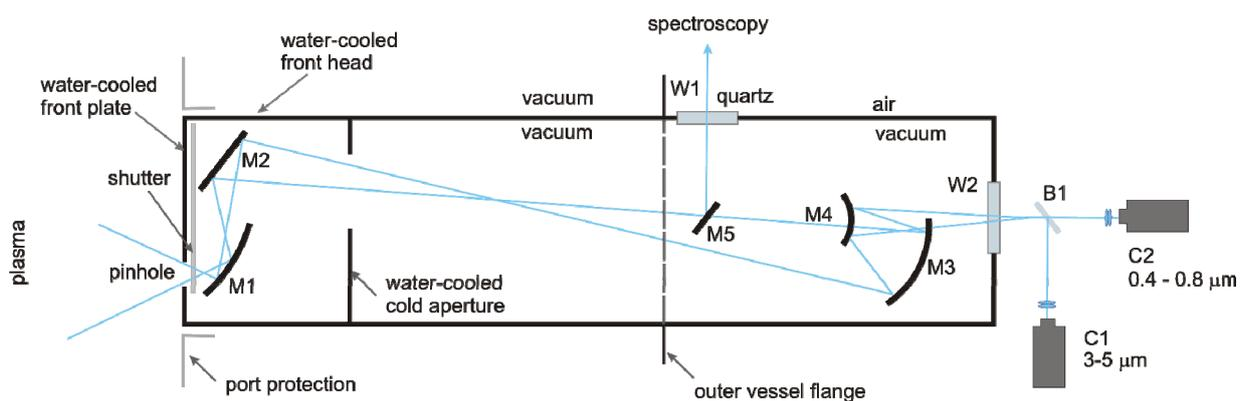
Figure 2. Functional sketch of the IR/VIS endoscope with its main components: M1 - heated, ellipsoid mirror, M2 - flat mirror, M3, M4 - off-axis Cassegrain mirrors, M5 - flat mirror, W1-W3 - windows, B1 - dichroic beam splitter, C1 - fast, infrared camera, C2 - visible camera.
