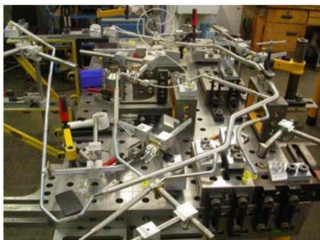
Fig.3 Cooling circuit on the welding facility during production at ITZ, IPP-GAR.
