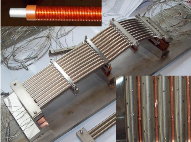
FIG. 3. Mock-up Rogowski coil section (centre) consists of 10 individually 3D shaped rods (top left) with tightly wound wire placed into thin SS tubes for ECRH protection with 0.7 mm holes for outgassing and copper rails clamped between rods (bottom right) to improve cooling
