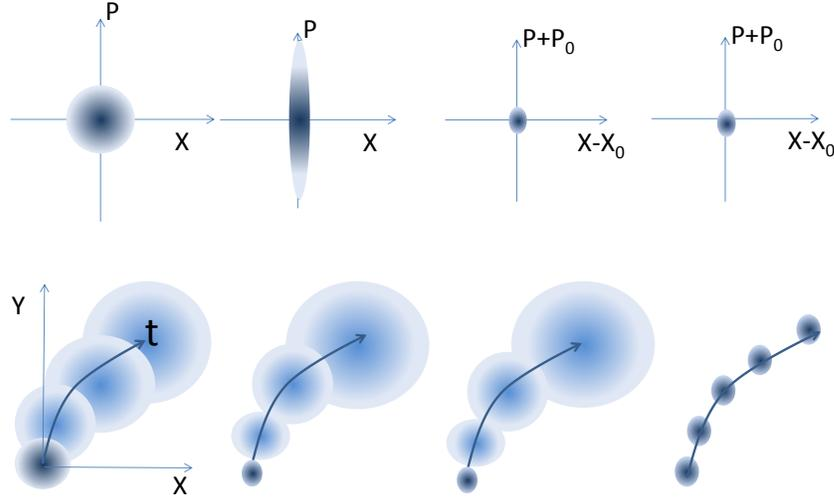
**Fig. 1 Trajectories for various quantum states.** Upper row - quantum states of the system, lower row - trajectories. From left to right: coherent state, squeezed state, EPR state with positive mass(frequency), EPR state with negative mass (frequency)
