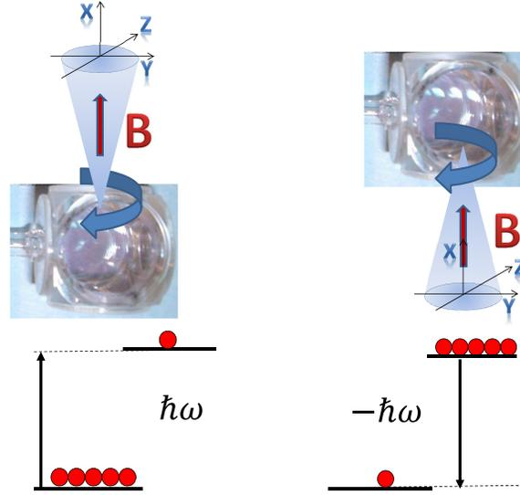
**Fig. 2** Collective spin oscillators with an effective positive and negative masses. The ensemble on the left is polarized along the magnetic field direction. Excitation of the ensemble from a fully polarized state corresponds to the precession of the spin in the field with positive magnetic energy. The ensemble on the right is polarized in the opposite direction and its excitation corresponds to the precession with a negative magnetic energy, or an effective negative mass.
