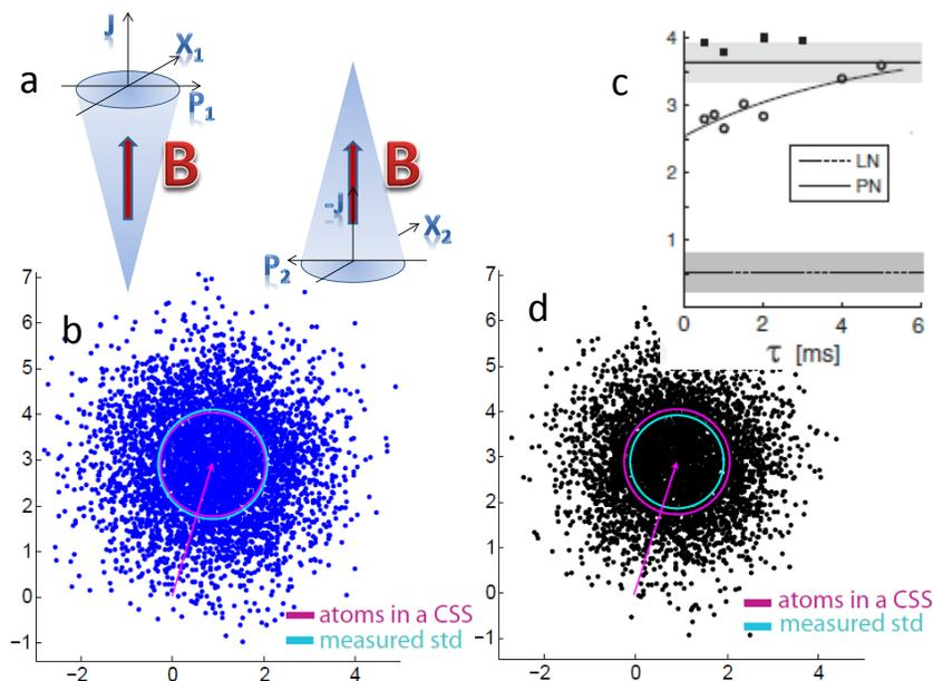
**Fig. 3 Trajectory beyond the standard quantum limit.** (a) Two magnetic oscillators (b) Results of a series of measurements of 1 msec evolution of one spin in the reference frame of the other spin for both spins for uncorrelated spins (c) The EPR variance of the entangled state of the two spin oscillators (d) Same as in (b) but for an entangled state of the two oscillators
