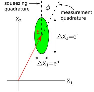
FIG. 1: Phasor diagram of a squeezed state ( $\Delta X_1 \Delta X_2 \geq 1$ ). The factor  $r$  describes the degree of squeezing and anti-squeezing for a pure state and  $\phi$  describes the mismatch in angle between the squeezing and measurement quadratures. For application in a GW detector, phase squeezing is injected to the anti-symmetric port.
