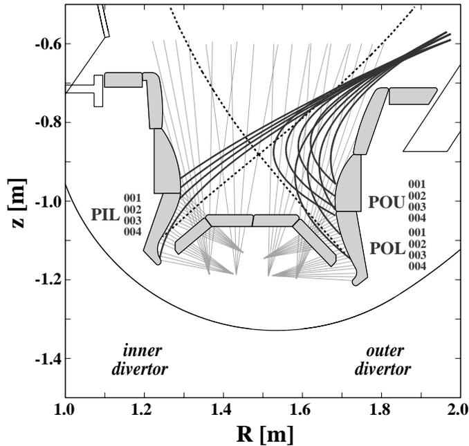
**Figure 1.** A subset of 12 toroidal lines of sight (thick black lines) in the ASDEX Upgrade Divertor II projected into a poloidal plane; the outer and inner divertor areas are covered to allow for spatially resolved velocity measurements. The poloidal lines of sight (thin grey lines) probe the X-point region and the area in front of the target plates with high spatial resolution.
