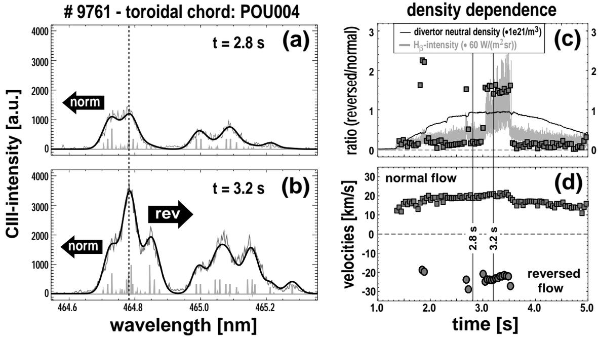
**Figure 2.** Spectroscopic observation of  $C^{2+}$ -flow-reversal in toroidal chord POU004 (near separatrix; comp. Fig. 1b) in an L-Mode density ramp: (a) blue-shifted CIII-spectrum ( $t=2.8$  s; attached), (b) superposition of additional red-shifted CIII-component (reversed flow) onto blue-shifted one ( $t=3.2$  s; detached), (c) ratio (reversed/normal), divertor neutral density and  $H_{\beta}$ -emission (outer separatrix) as detachment monitor and (d) resulting  $C^{2+}$ -flow-velocities
