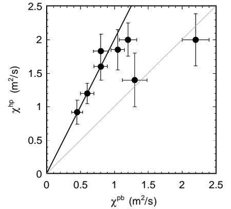
**Figure 3.** Heat diffusivities from power balance and heat pulse analyses.
