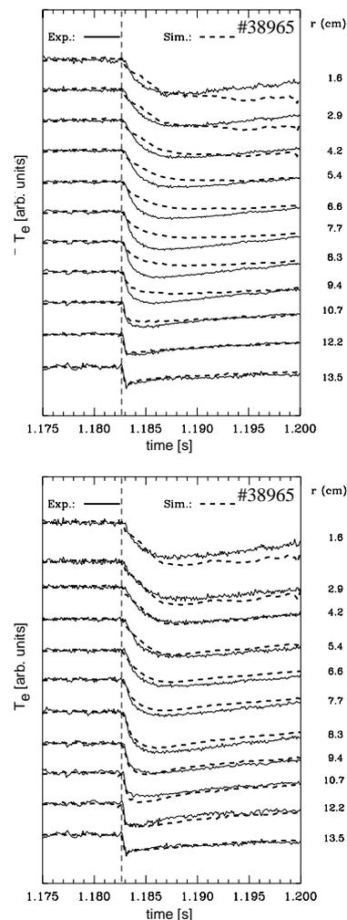
**Figure 2.** Comparison of the simulated and measured electron temperature evolution for a large cold-pulse using two different models as described in the text.
