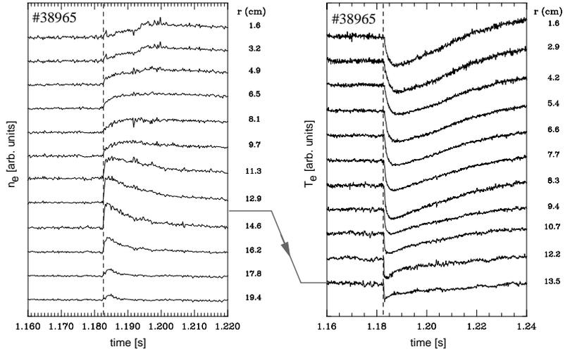
**Figure 1.** Electron density and temperature evolution at different radii of a cold-pulse induced by carbon injection (dashed line).
