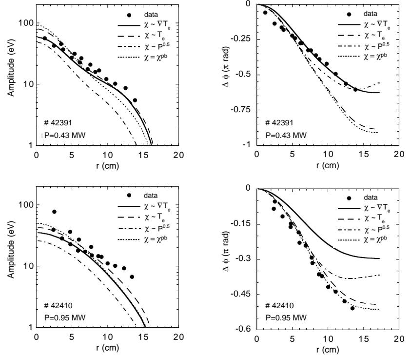
**Figure 4.** Comparison between measured and simulated amplitude and phase profiles. ECH power is depicted in the center.
