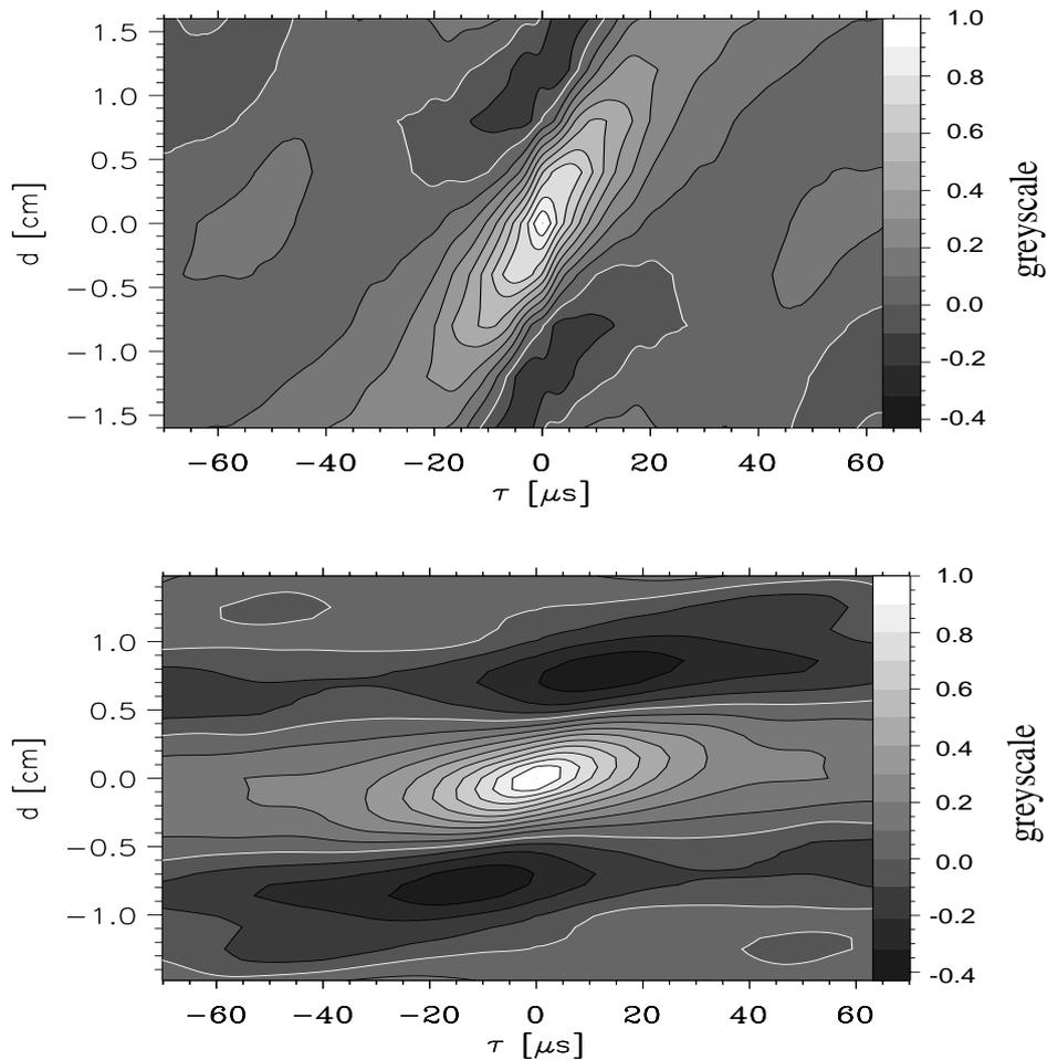
**Figure 1.** Poloidal-temporal correlation function of floating potential fluctuations in the SOL of the Wendelstein 7-AS stellarator (top) and of simulated fluctuation data (nonlocal model, bottom).
