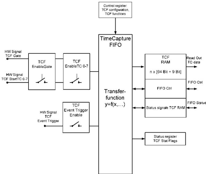
Fig. 2: Structure of the TCF device
