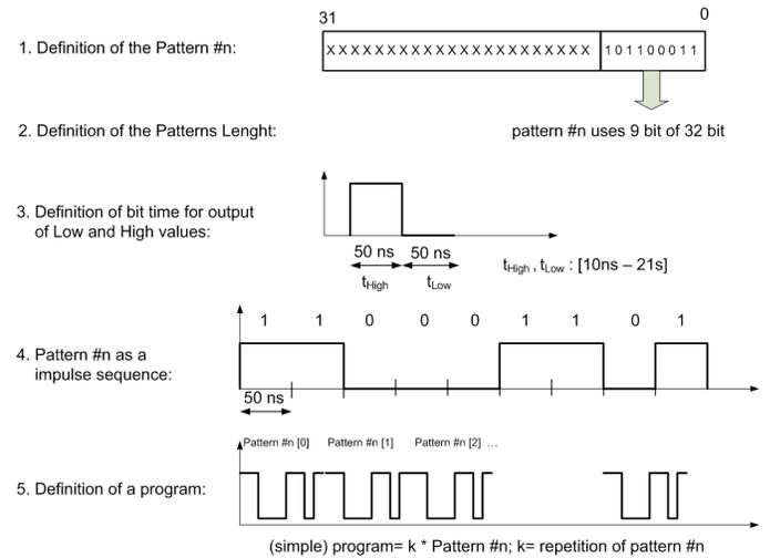
Fig. 3: Definition of a simple impulse program consisting of one pattern
