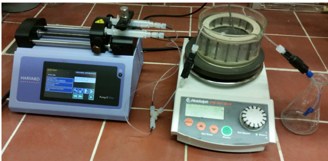
Image 1: Setup of gold(I)-catalyzed glycosylations in flow.
