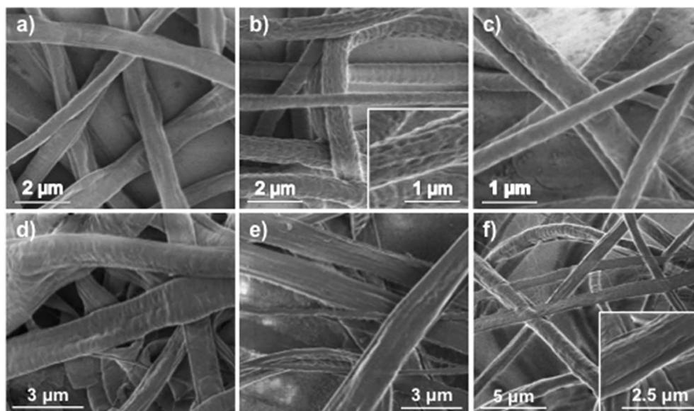
Fig. 2 SEM micrographs of the prepared electrospinning scaffolds. (a) PCL without R6G, (b) PCL, (c) PCL<sub>L</sub>, (d) PM, (e) PM<sub>L</sub>, and (f) PM<sub>CT</sub>. See nomenclature in Table 2. Insets show a magnification of the respective samples.
