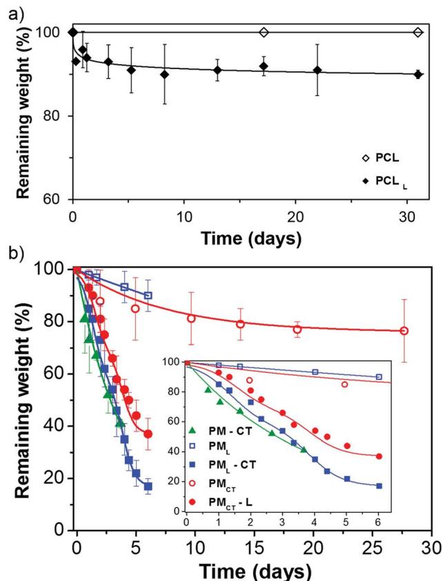
Fig. 4 Weight loss of the nanofibers by enzymatic degradation versus time for (a) PCL and PCL<sub>L</sub> scaffolds and (b) PCL/coPEA 70/30 scaffolds (PM samples).
