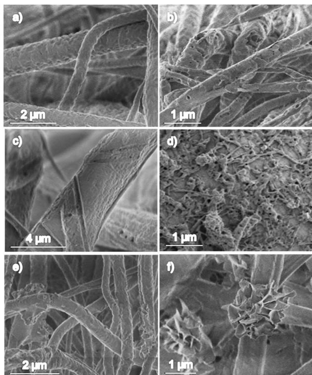
Fig. 5 SEM micrographs of: (a) PCL scaffold after 412 h of immersion in DPBS medium, (b) PCL<sub>L</sub> enzyme loaded scaffold after 198 h of immersion in DPBS medium. (c) Sample PM-CT after immersion in  $\alpha$ -chymotrypsin medium for 16 h and (d) 88 h. (e) Sample PM<sub>L</sub>-CT after immersion in  $\alpha$ -chymotrypsin medium for 48 h. (f) Sample PM<sub>CT</sub>-L after immersion in lipase medium for 48 h.
