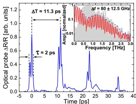
FIG. 4. (Color online)  $\Delta R/R$  of the optical probe signal in the QDs, provided by the multiple reflections of a single THz pulse in the QD sample. Inset: amplitude Fourier spectra of the isolated first  $\Delta R/R$  modulation pulse around 0 ps (dashed line), and of the full multipulse sequence. Background: amplitude spectrum of a single THz pulse.
