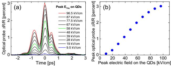
FIG. 3. (Color online) (a)  $\Delta R/R$  of the optical probe signal in the QD sample, under influence of the incident THz pulses with variable peak field strength. (b) Peak values of  $\Delta R/R$  of the signals from (a), as a function of peak THz field on the QDs.
