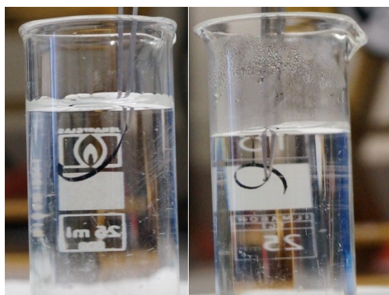
Figure S4: Left: Membrane in water at 22 °C (left) and at 60 °C (right).
