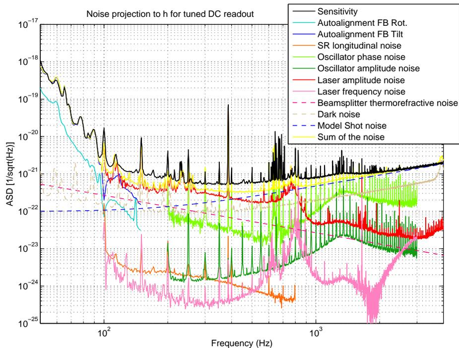
**Figure 2.** Noise budget of the tuned DC readout configuration.
