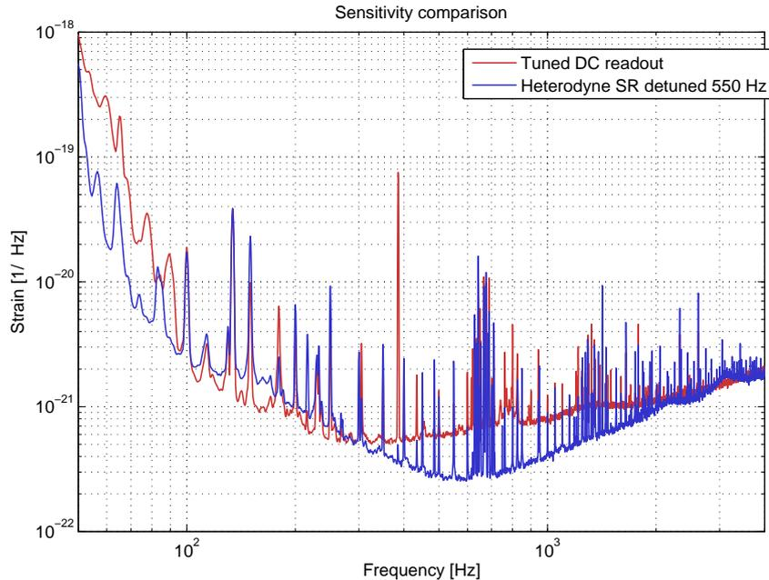
**Figure 1.** Sensitivity comparison between the preliminary tuned DC readout configuration and the heterodyne readout used during S5 and Astrowatch.
