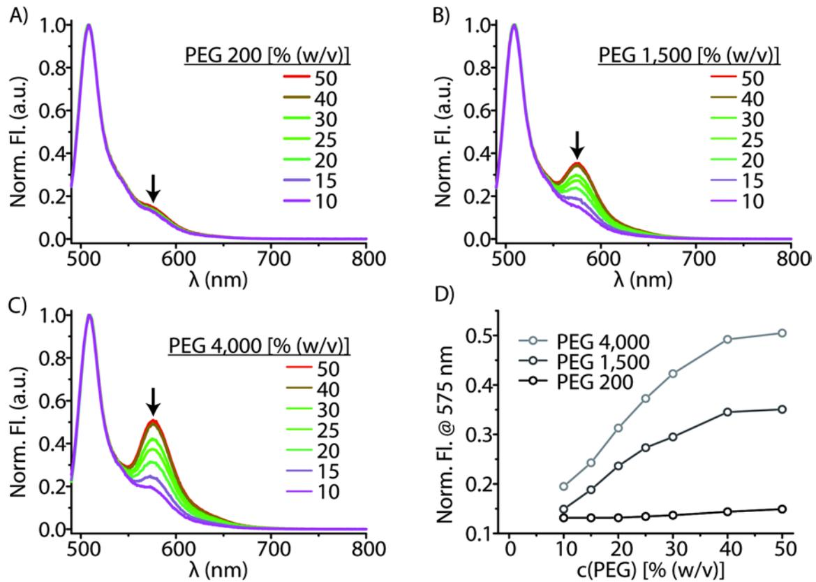
A-C) Starting from a *hsImportin- $\beta$ -sfGFP Q220AzF-Fl.-545* solution containing a concentration of 50% PEG of the indicated molecular weight buffer is added stepwise. Between each addition fluorescence emission scans were acquired. Fluorescence was normalized for each spectrum setting the highest peak to 1.0. D) Emission intensities at 575 nm of panels A-C were plotted against PEG concentration.
