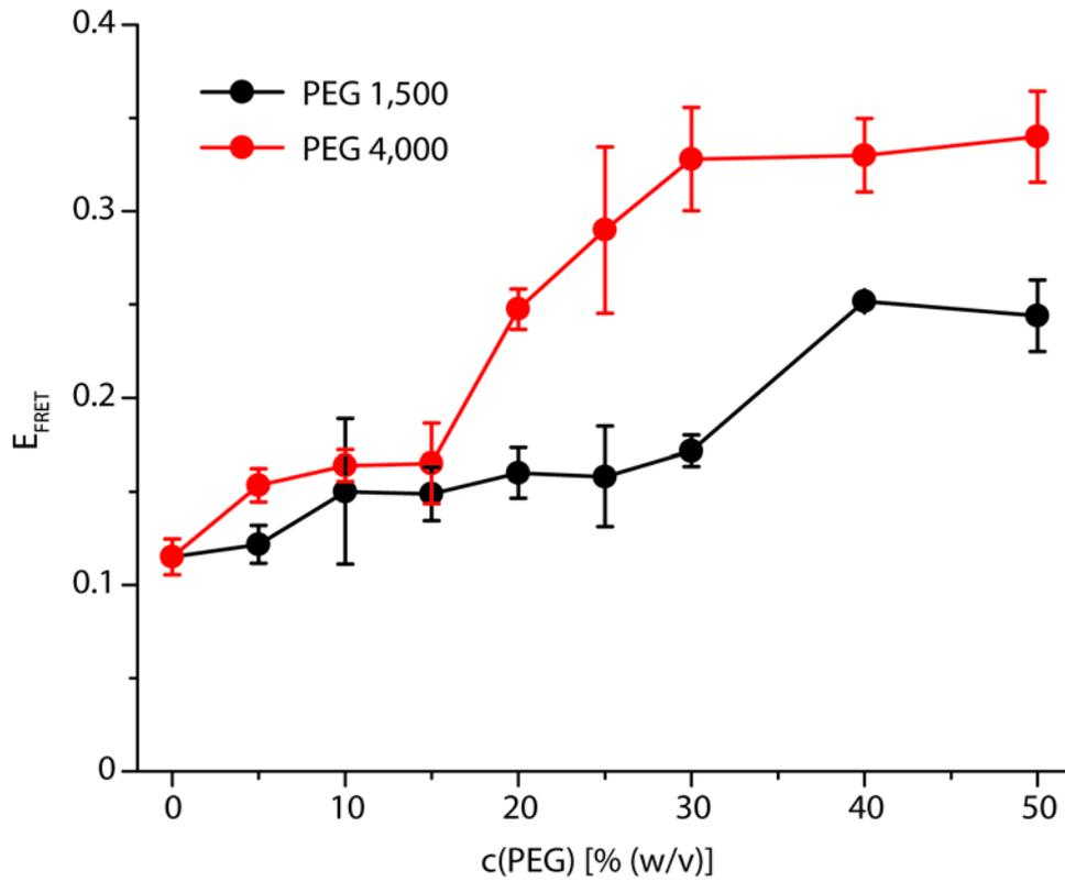
Addition of PEG 1,500 or PEG 4,000 increases relative FRET efficiency in *hsImp $\beta$ -sfGFP Q220AzF-Fl.-545* determined by donor fluorescence lifetime measurements. Error bars represent standard error of the mean.
