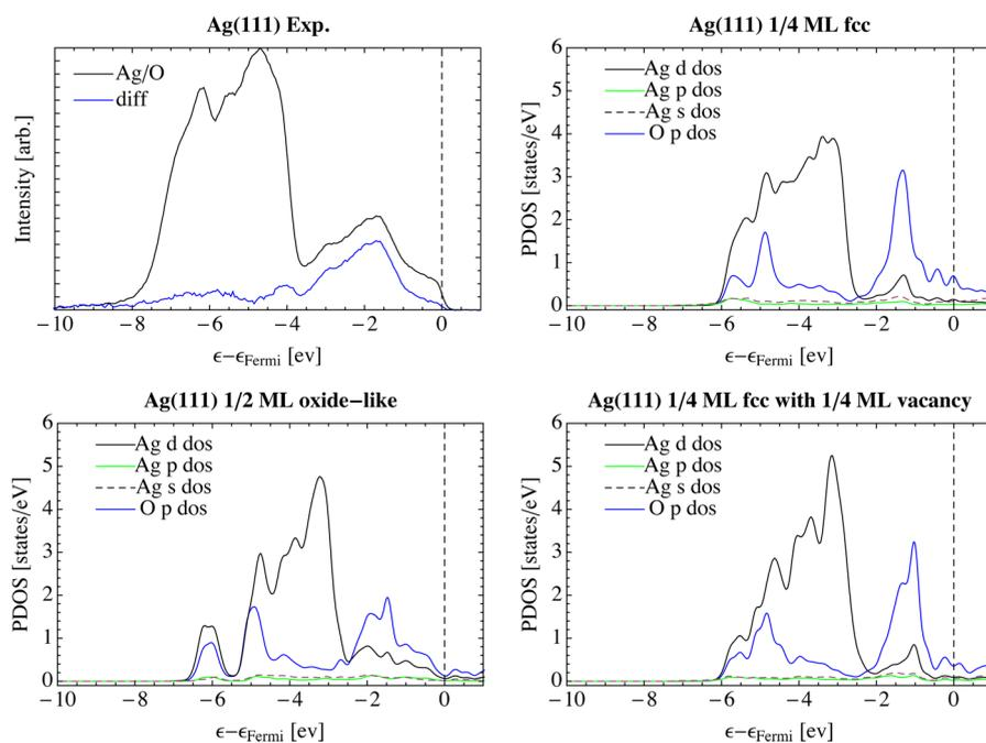
**Figure 2.** In situ valence band spectrum of a Ag(111) surface under  $4 \times 10^{-4}$  mbar  $O_2$  at 423 K (upper left). The blue curve shows the difference between the in situ spectrum and that of clean silver. Calculated PDOS of oxygen and that of its nearest neighbor silver atom when oxygen is adsorbed on the fcc site (upper right), in an oxide-like layer (lower left), and adjacent to a surface vacancy (lower right) on the Ag(111) surface.
