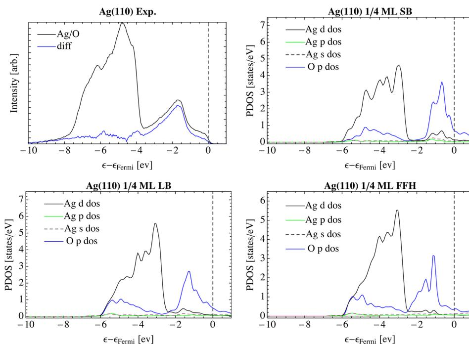
**Figure 1.** In situ valence band spectrum of a Ag(110) surface under  $1 \times 10^{-4}$  mbar  $O_2$  at 423 K (upper left). The blue curve shows the difference between the in situ spectrum and that of clean silver. Calculated PDOS of oxygen and that of its nearest neighbor silver atom when oxygen is adsorbed on the short bridge (upper right), long bridge (lower left), and 4-fold hollow sites (lower right) on the Ag(110) surface.
