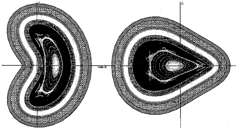
**Fig. 1:** Cross section of plasma and coils at  $\langle\beta\rangle = 5\%$ . Left:  $\phi = 0^\circ$ , right  $\phi = 36^\circ$ . Width of blanket and shield is 1.2 m at all locations around the torus.
