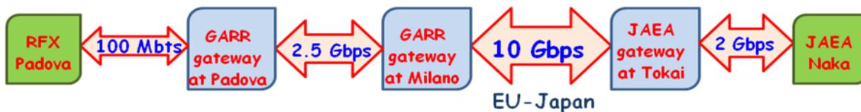
Fig. 1: RFX to JAEA Network connection.
