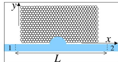
FIG. 3: Schematic view of a zigzag-edge graphene ribbon with a side tunnel contact to a quasi-one-dimensional conducting wire connecting electron reservoirs 1 and 2. The contact is assumed point-like, that is its size is much bigger than the interatomic distances, but smaller than the electronic mean free paths in both wire and graphene.
