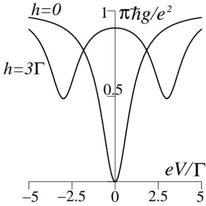
FIG. 4: Zero-temperature conductance  $g$  vs. bias voltage  $V$  for spin-degenerate ( $h = 0$ ) and spin-split ( $h = 3\Gamma$ ) edge state in graphene. In the latter case the two minima manifest the spin-filtering effect when the contribution of one of the spin species resonantly vanishes.
