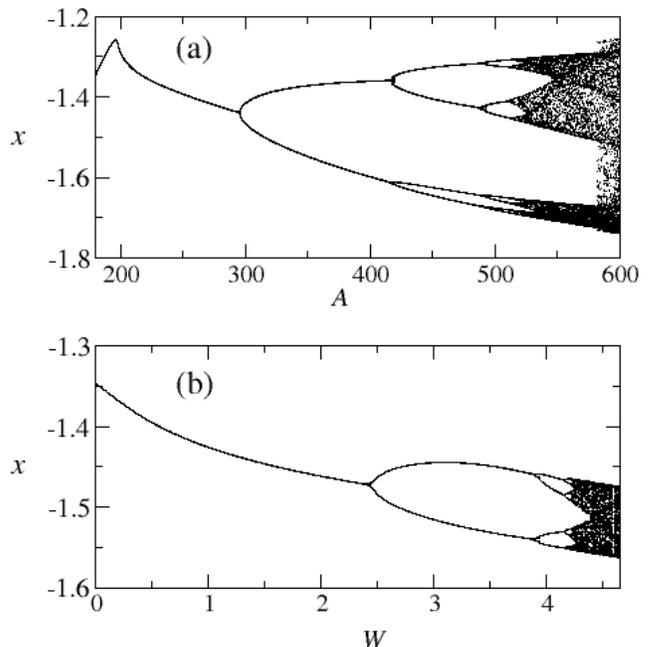
FIG. 4: Bifurcation diagrams showing the  $x$ -coordinates of the attractor at time  $t \bmod T = 0$  (a) as a function of the parameter  $A$  in the absence of gravity and (b) as a function of  $W$  when  $A = 180$ . The unspecified parameters are the same as in Fig. 2(b).
