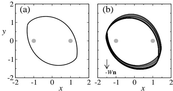
FIG. 3: (a) Periodic attractor corresponding to  $W = 0$  and (b) strange attractor corresponding to  $W = 40/9$ . The gray dots represent the point sources. The unspecified parameters are the same as in Fig. 2(b).
