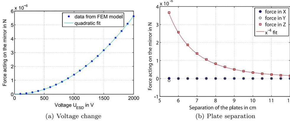
**Figure 5.** Figure (a) shows the force on the mirror for different voltages. The relative position of mirror and ESD is the position with the optimal force. (b) Shows how the force depends on the plate separation (assuming that the mirror is at the ideal operating position).
