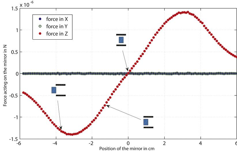
**Figure 4.** Longitudinal force on the mirror, versus relative longitudinal position of mirror and ESD. The  $x$ -axis shows the relative distance between the mirror center and the center of the capacitor plates.
