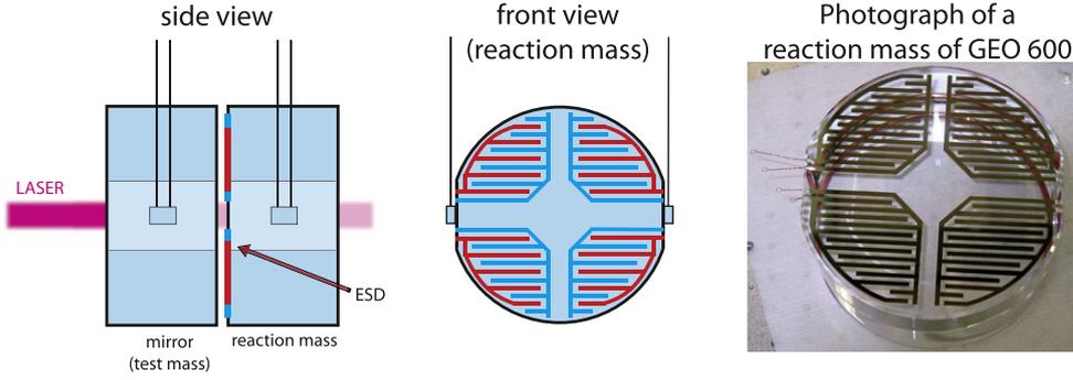
**Figure 1.** Left and center: schematic drawing of a conventional ESD setup. The ESD setup consists of four independent ESD comb-shaped electrode pairs on a single reaction mass. The anodes are colored in red, the cathodes are colored blue. The center of the reaction mass is kept free so that a laser beam can pass without significant clipping. Right: photograph of a reaction mass of GEO 600.
