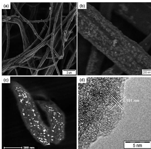
Fig. 2 Electron micrographs of the electrospun poly(styrene-*co*-vinylphosphonic acid) P(S<sub>0.90-co</sub>-VPA<sub>0.10</sub>) fibers after ceria crystallization: (a) and (b) SEM micrographs at different magnifications, (c) TEM dark-field micrograph of a microtomed section the hybrid fibers, and (d) high-resolution TEM image.
