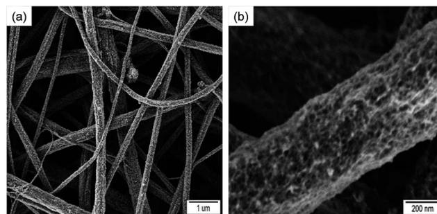
Fig. 4 SEM micrographs of the electrospun poly(styrene-*co*-vinylphosphonic acid) P(S<sub>0.99-co</sub>-VPA<sub>0.01</sub>) fibers after TiO<sub>2</sub> crystallization: (a) general view, (b) higher magnification of the fiber surface.
