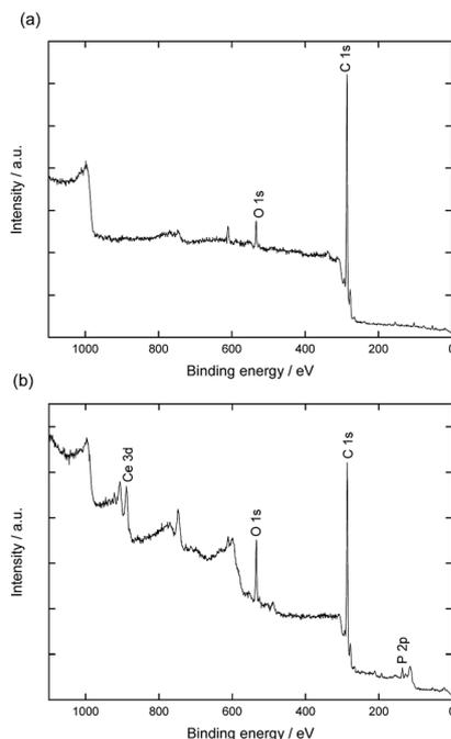
Fig. 3 XPS spectra of the electrospun poly(styrene-*co*-vinylphosphonic acid) P(S<sub>0.96-co</sub>-VPA<sub>0.04</sub>) fibers (a) before and (b) after ceria crystallization.
